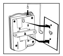
Fig. 6 - Wall mounting installation.
